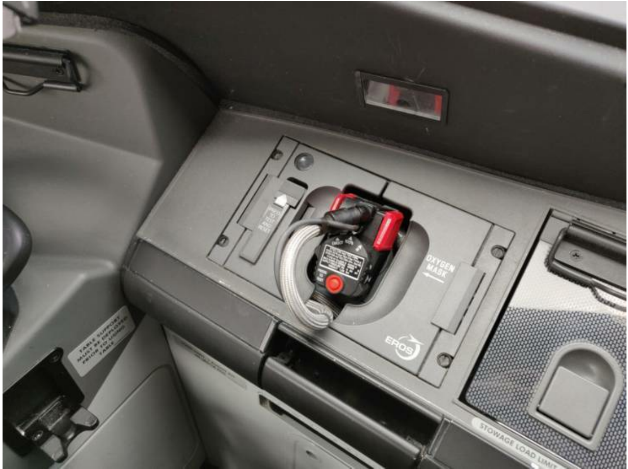
The oxygen mask is easily accessible for quick donning.
