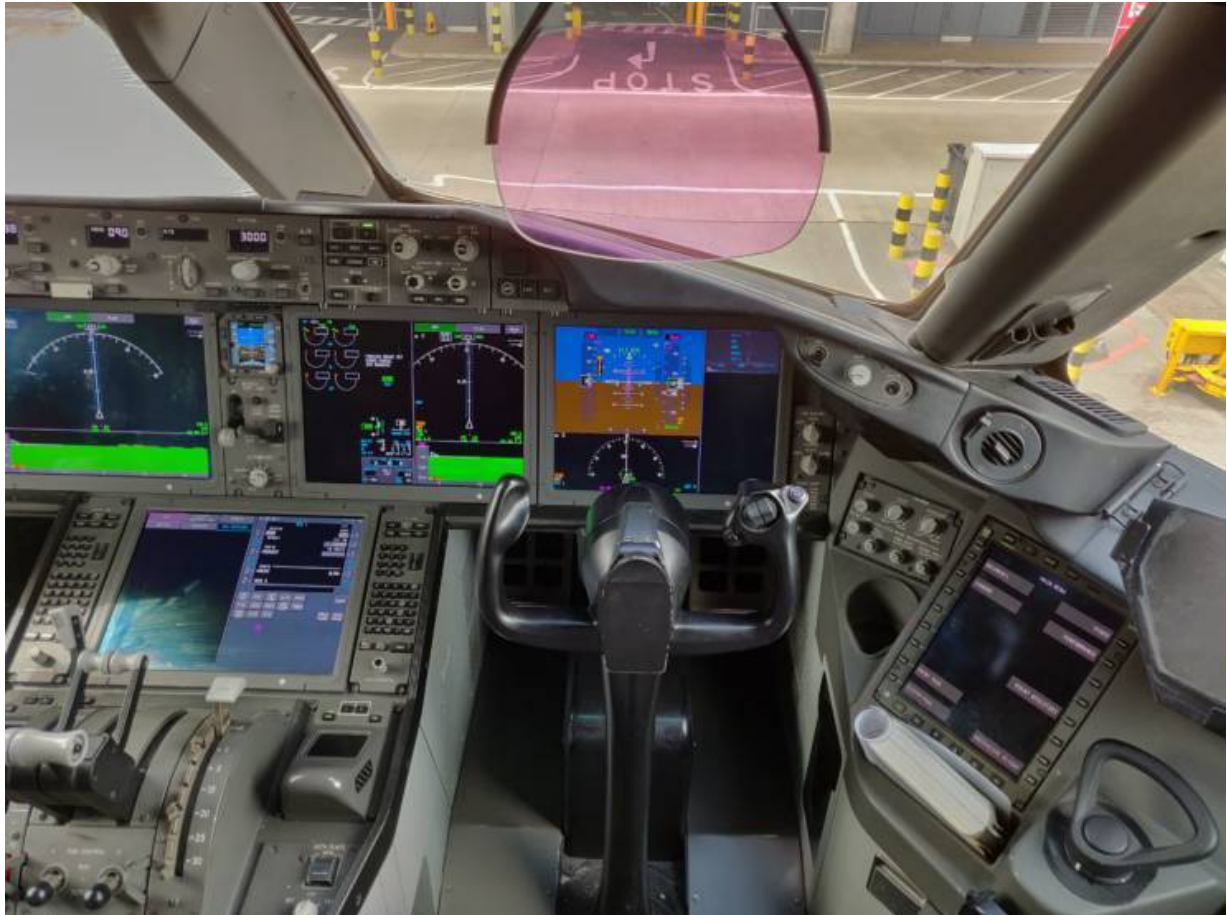
The control column sits between the pilot's legs.
