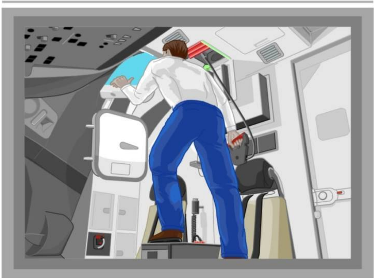
The escape hatch is in the roof of the flight deck. (Image courtesy Boeing)
