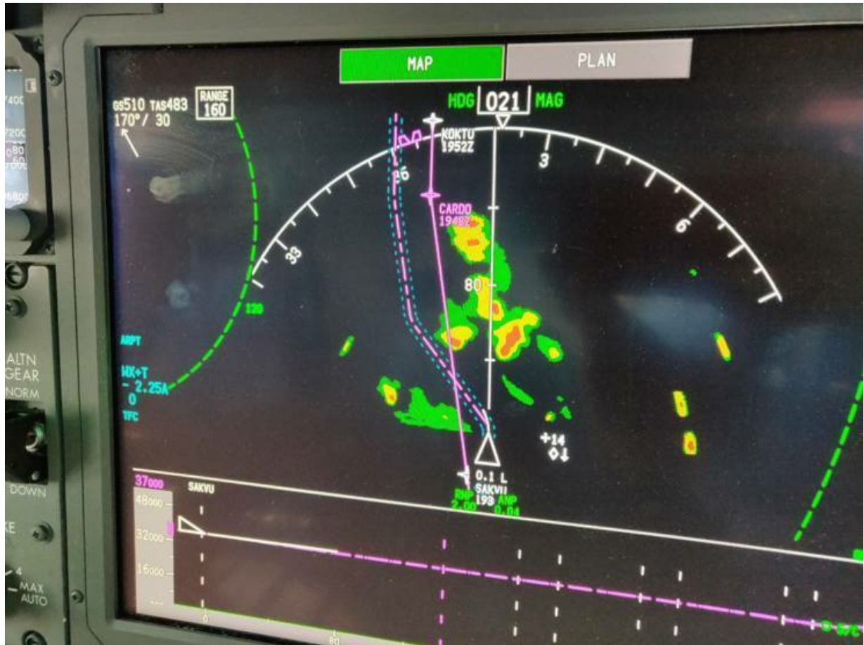
The ND shows the planned route (solid magenta), weather returns and actual route (dotted magenta).
