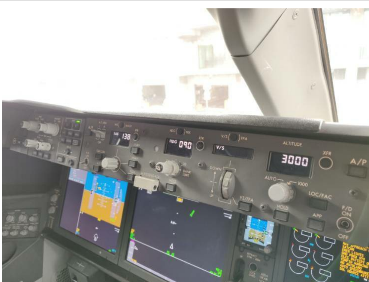
The glare shield panel controls the autopilot.
