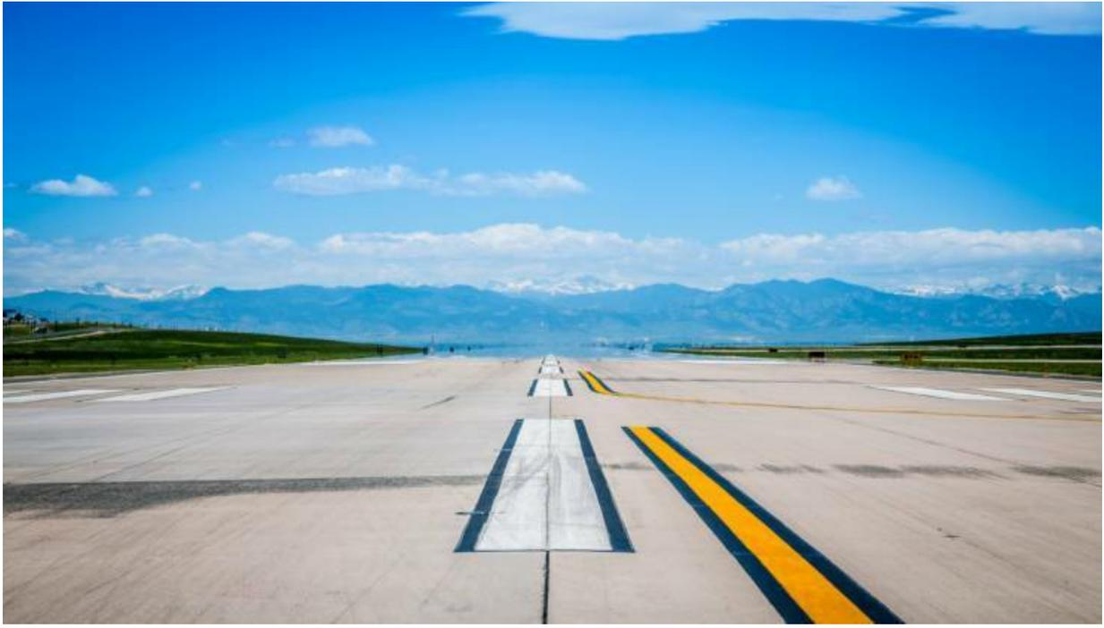
The runway slope affects takeoff performance. The greater the upslope, the greater the engine power needed.
