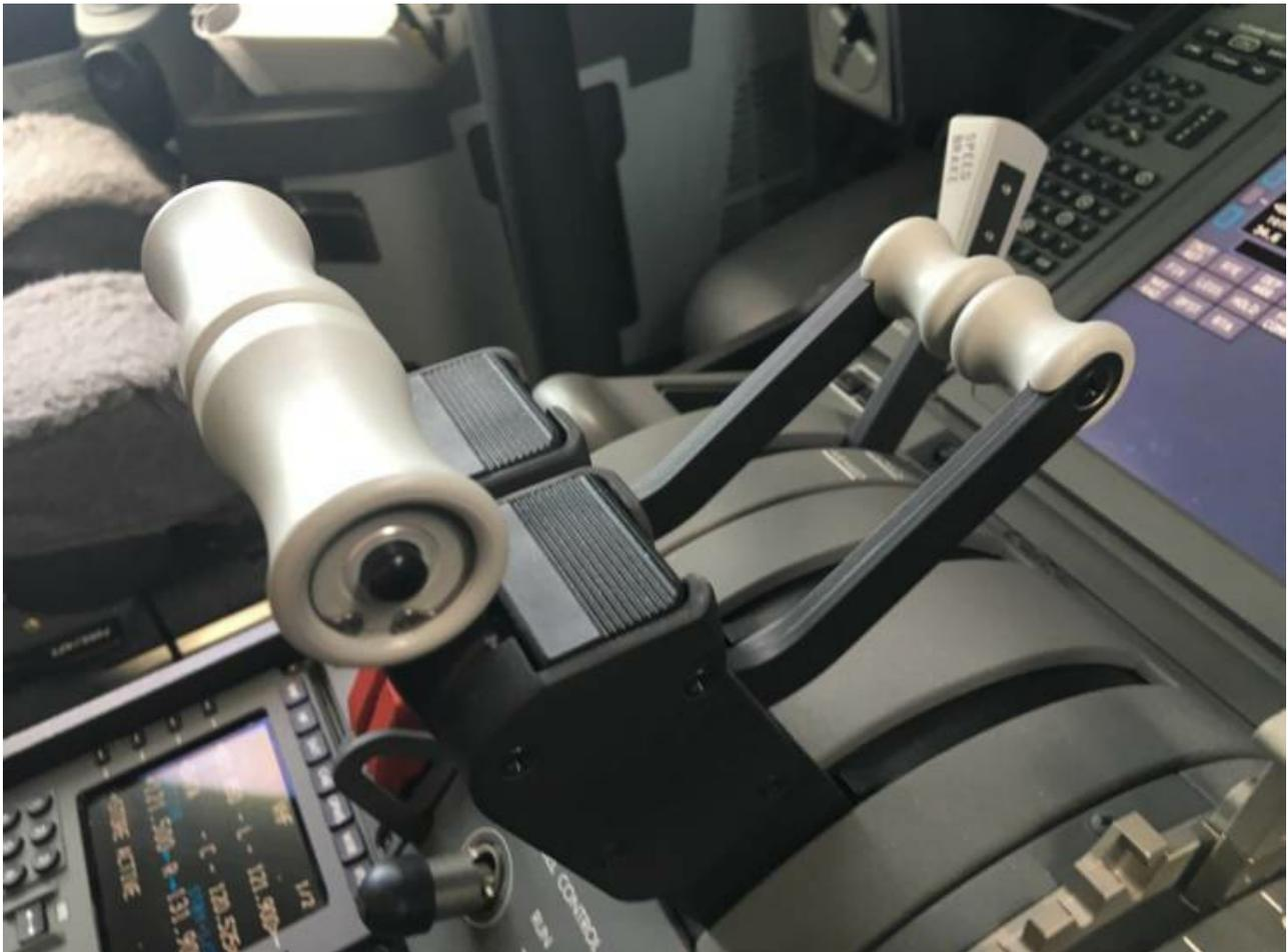
The autothrottle disconnect button on the side of the thrust lever. (Photo Charlie Page/The Points Guy)
