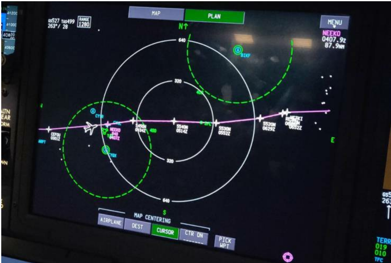
Gander, CYQX in the centre of the lefthand green circle, is ideally situated as an ETOPS alternate. (Image by Charlie Page/The Points Guy)
